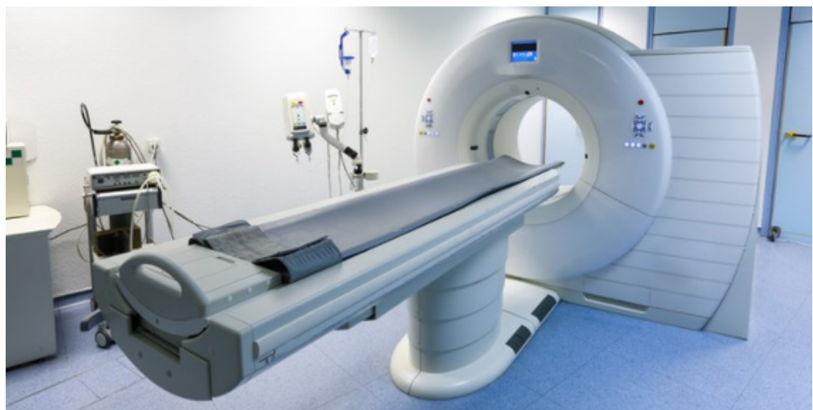
Figure 1: A tomography device similar to a medical use for porosity analysis.
